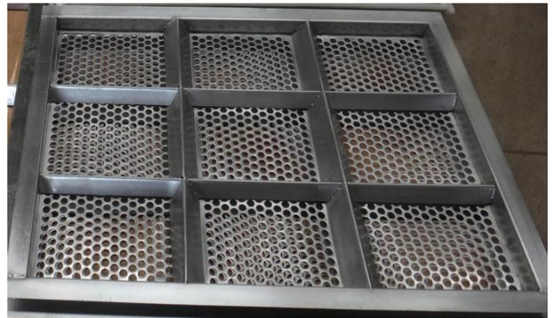
The side door gyrotory screener deck is one combination structure that consist of screener mesh , self-cleaning ball and support deck frame. The screener mesh be fixed on screener ball tray directly.
