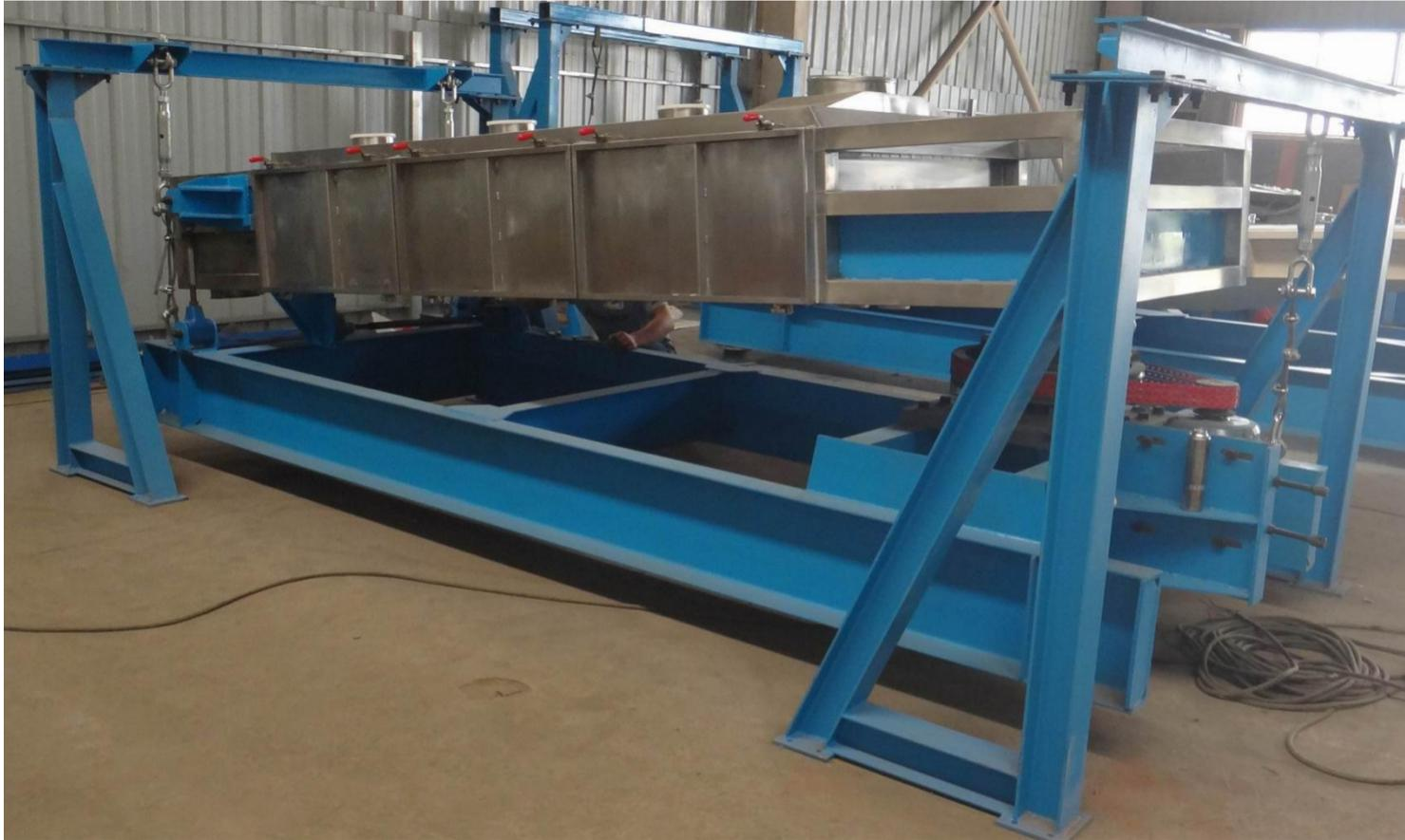
MHG series gyrotory screens is similar with M serial gyrotory screen such as the screening principle, screening efficiency and application, just except the screen deck structure.
