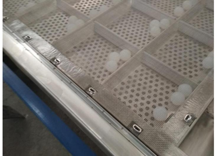
The gyrotory screener deck is one combination structure that consist of screener mesh , self-cleaning ball and support deck frame.
