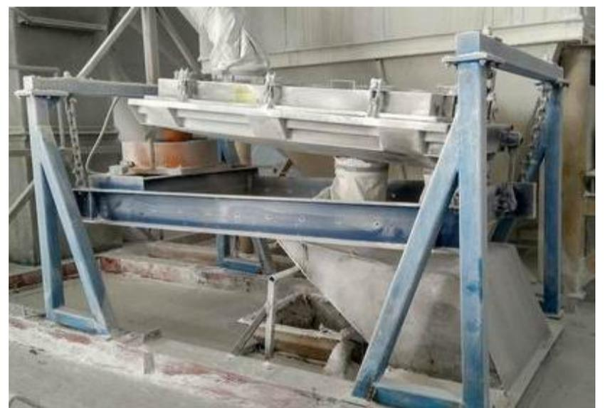
MH Gyrotory Screen at Sugar Screening site
