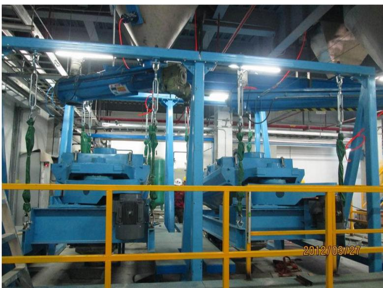
MH Gyrotory Screen at PVC screening site
