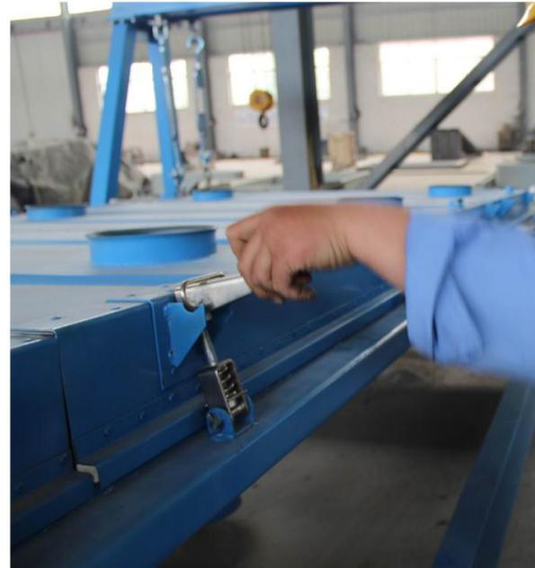
The fast clamp for top cover is adjustable, and it is easy to open and fasten
