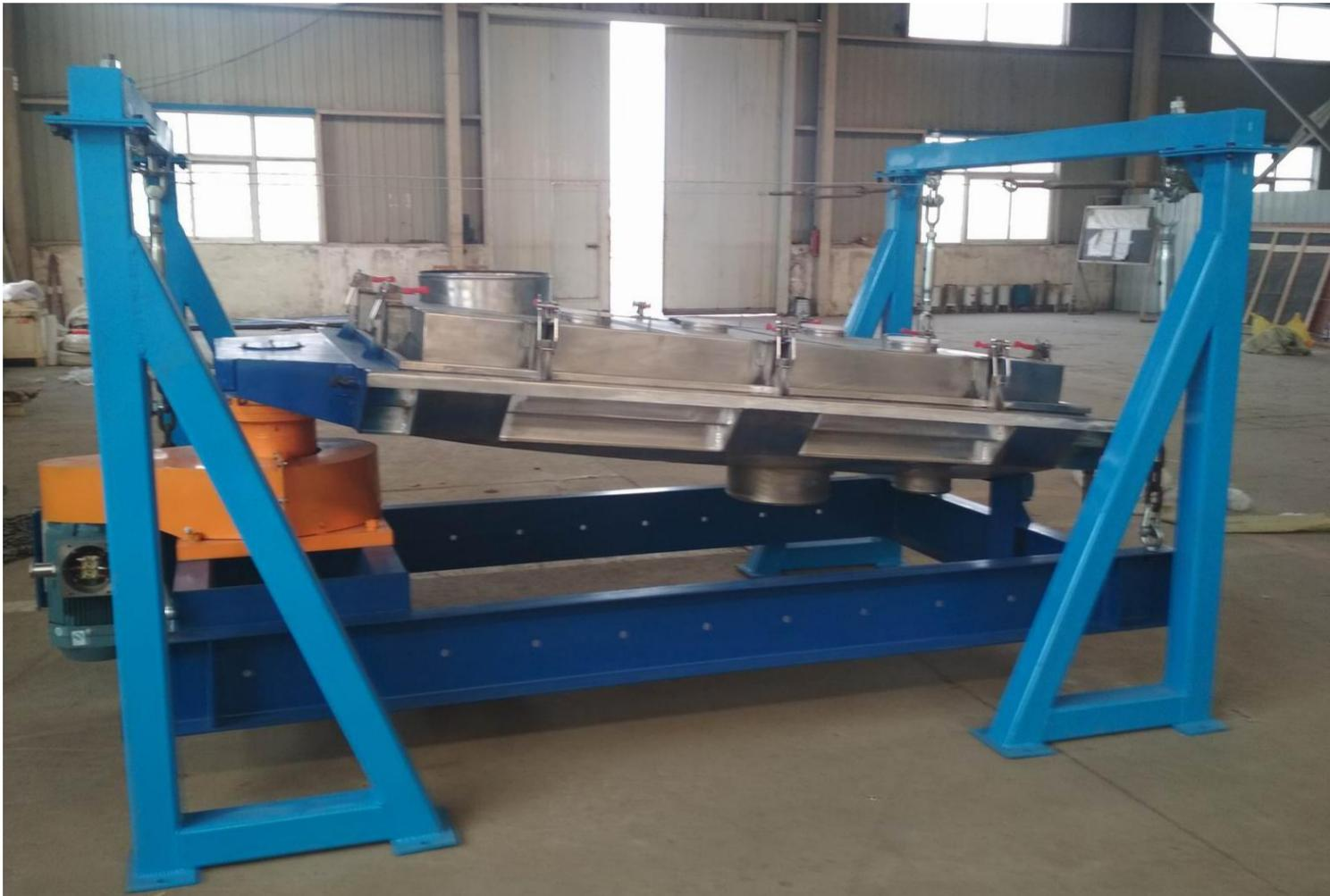
MH gyrotory screener adopt suspension installation method, and because the gyrotory screener motion path is one reciprocating gyrotory month on one almost horizontal plane, there is no vertical vibration about the complete screening equipment, so this model screener do not need heavy and strong foundation, so it could save the building structure cost for customer.
