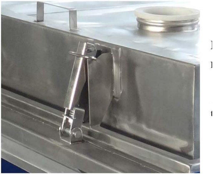
The fast clamp for top cover is adjustable, and it is easy to open and fasten
